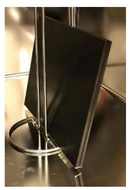
Climate chamber Temperature Relative humidity Air velocity at the surface of the specimen Air change rate (n) Material load (L) Area specific air flow rate (q) 113 L Polished stainless steel 23°C  $\pm$  1°C 50% RH  $\pm$  5% RH 0.1 – 0.3 m/s 1.0 h<sup>-1</sup>  $\pm$  0.05 h<sup>-1</sup> 1.0 m<sup>2</sup>/m<sup>3</sup> 1.0 m<sup>3</sup>/m<sup>2</sup>h
